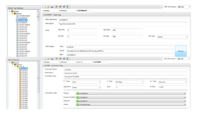
The Master Tag Database allows the user to create, edit and save all details relevant to a unique data tag or a complete controller.
